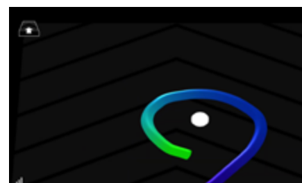
Sky View Mode: Displays the endoscope model obliquely from above the foot section of the patient
